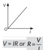
So, the slope of V-I graph at any point represents the resistance of the given conductor. As graph is a straight line, so it is clear from the graph that  $V \propto I$ .
