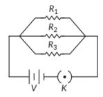
$$\frac{1}{R_{eq}} = \frac{1}{R_1} + \frac{1}{R_2} + \frac{1}{R_3}$$
