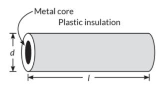
Plastic insulation surrounds a wire having diameter d and length I as shown above. A decrease in the resistance of the wire would be produced by an increase in the
