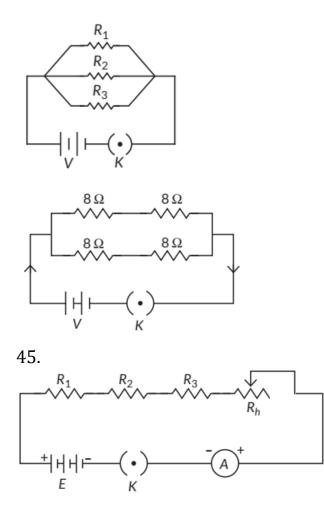
Change the positions of ammeter and note the reading of ammeter each time. You will find that all the reading obtained are same. So, the value of the current in the ammeter is the same, independent of its position in the electric circuit. It means that in this circuit (series combination) the current is the same in every part of the circuit. Precautions:
