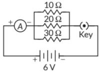
(a) Given, voltage of the battery =  $2\mathrm{V}+2\mathrm{V}+2\mathrm{V}=6$  V Current through 10  $\Omega$  resistance,
