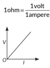
V-I graph for an ohmic conductor can be drawn as given in figure. Important feature of V-I graph are:
