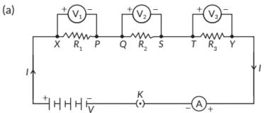
Given figure shows, the series combination of three resistors  $R_1$ ,  $R_2$  and  $R_3$  connected across a voltage source of potential difference V.
