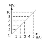
Hence, the value of current for V = 10 volts is 5 amperes (or 5 A). From Ohm's law, V = IR,
