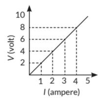
10. V-I graph for a conductor is as shown in the figure
