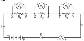
Given figure shows the series combination of three resistors  $R_1$ ,  $R_2$  and  $R_3$  connected across a voltage source of potential difference V. Let current I is flowing through the circuit.  $V_1$ ,  $V_2$  and  $V_3$  are the potential differences across resistors  $R_1$ ,  $R_2$  and  $R_3$  respectively. Since, the total potential difference across a combination of resistors in series is equal to the sum of potential difference across the individual resistors.
